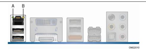
Figure 2. LAN Connector LEDs
